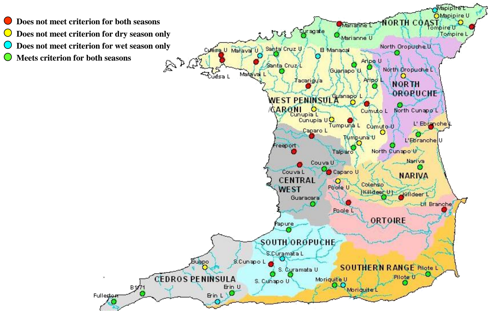
Figure 2.13: Map showing results for zinc in sediments of rivers in Trinidad and Tobago (not to scale) – Metal concentration compared to Canadian Sediment Quality Guidelines (1999)
